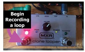
To begin recording a loop, press the "REC/DUB" footswitch. The light above the switch will turn red to indicate that you are recording.
