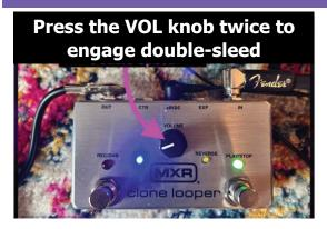
To double the speed instead of cutting it in half, press the volume knob twice and you'll see the blue light flashing a bit faster.
