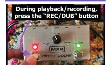
Press the "**REC/DUB**" during playback to begin overdubbing. It will flash red when it's in the middle of overdubbing.
