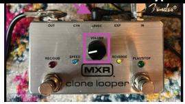
Hold the volume switch down while plugging in the power adapter to switch between True Bypass and Buffered Bypass.
