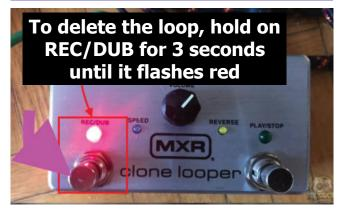
To clear an entire loop quickly with the MXR Clone Looper Pedal, press and hold the "REC/DUB" footswitch. To clear a single layer, simply press and hold the "PLAY/STOP" footswitch.
