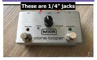
The CTL Jack is for the MXR Tempo Switch, which allows you to control the features of the pedal. The EXP Jack is for expression pedals, including universal pedals like the M-Audio EX-P.
